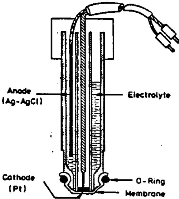
Fig. 2.3. Membrane covered polarographic oxygen sensor.
