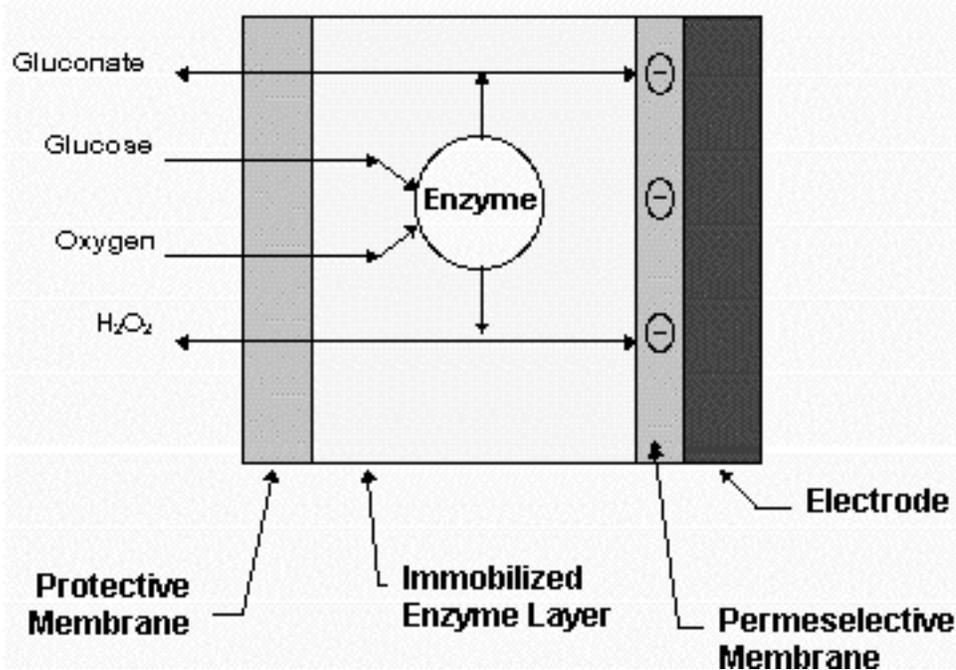
**Fig. 4.1. Overall structure of glucose biosensor.**
