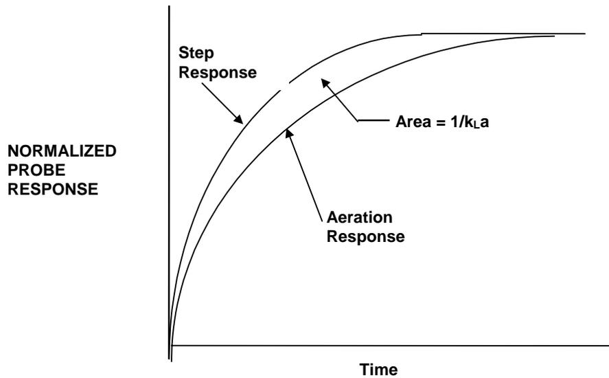
**Fig. 2.13. Measurement of  $k_L a$  by integral method.**
