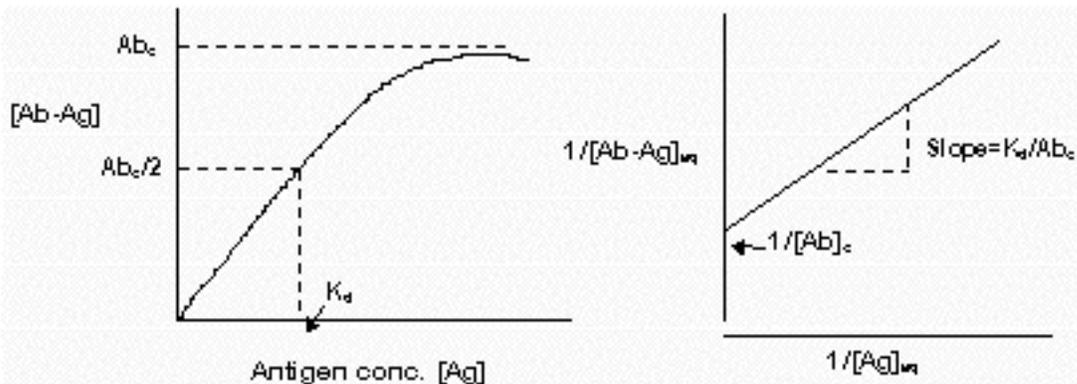
**Fig. 3.16. (a) Definition of  $K_d$ ; (b) graphical determination of  $K_a$ .**
