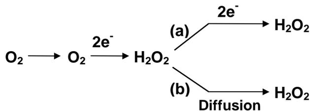
**Fig. 2.5. Alternative pathways of oxygen reduction at cathode surface.**
