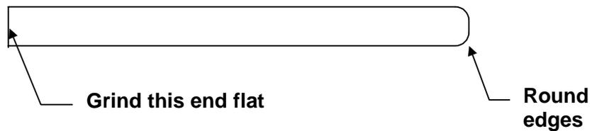
**Step 6.** Make a Ag/AgCl reference electrode by electrolytic chlorination of Ag wire.
