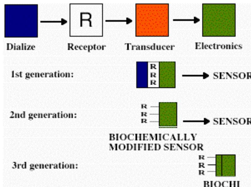
Fig. 1.14. Three biosensor generations (R: Bioreceptor molecule)
