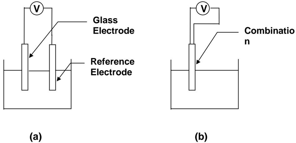
Fig. 2.16. Measurement setup for pH: (a) separate glass electrode and reference electrode; (b) a combination electrode.
