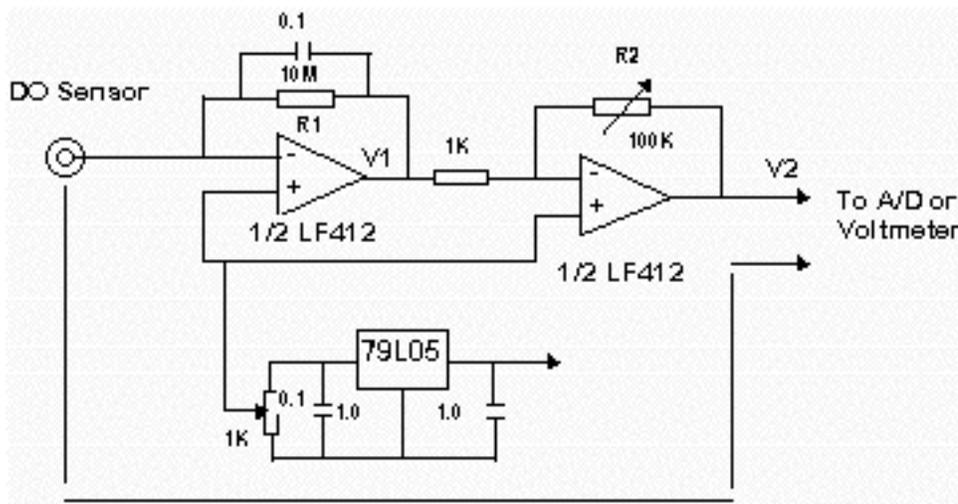
Fig. 2.11. Signal amplifier circuit for  $H_2O_2$  measurement.
