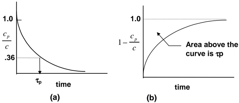
**Fig. 2.12. (a) Sensor response time measurement; (b) integral method for measuring the sensor time constant.**
