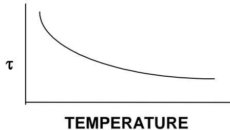
Fig. 2.10. Temperature dependency of DO sensor.
