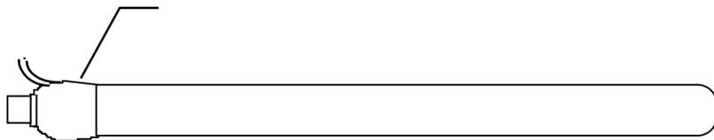
**Step 10.** Cut a 3/4" length of silicone tubing and place it in methyl chloroform for 2 min. The tubing swells. Cover the free end of the sensor assembly with a Teflon membrane and fix it tightly in place with the swelled silicone tubing. Make sure the membrane is tightly fit. Let the solvent evaporate.
