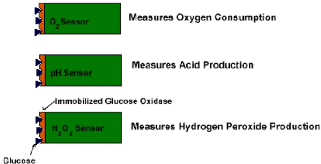
Fig. 1.3. Three possible transducers for glucose measurement.
