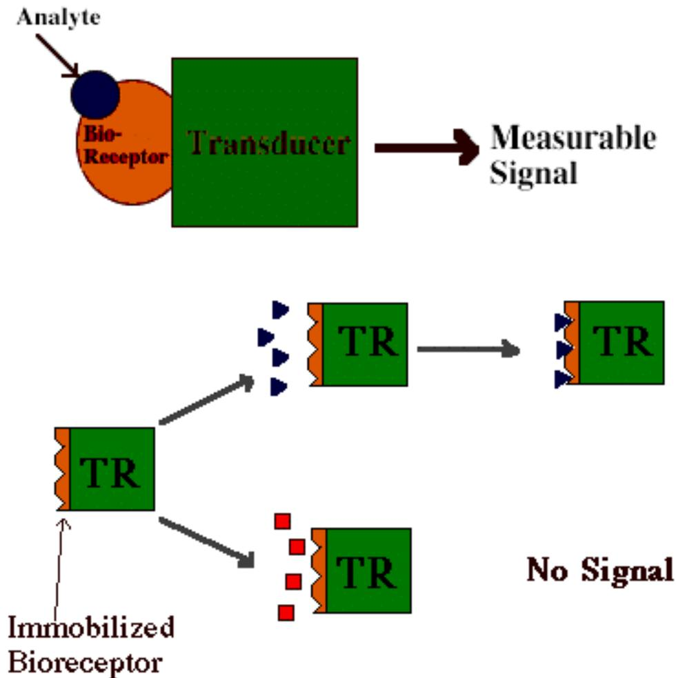
**Fig. 1.2. Specificity of biosensor (TR: transducer).**
