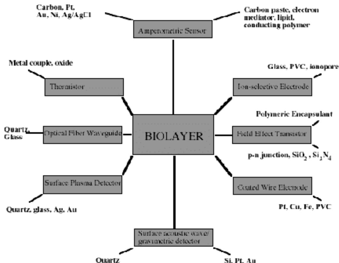
Fig. 1.12. Various biosensor configurations.
