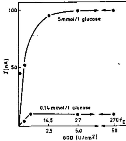
Fig. 4.4. Effect of enzyme loading factor on sensor output.
