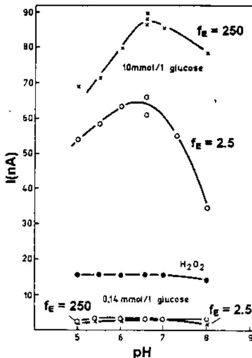
Fig. 4.6. Effect of pH on sensor output.
