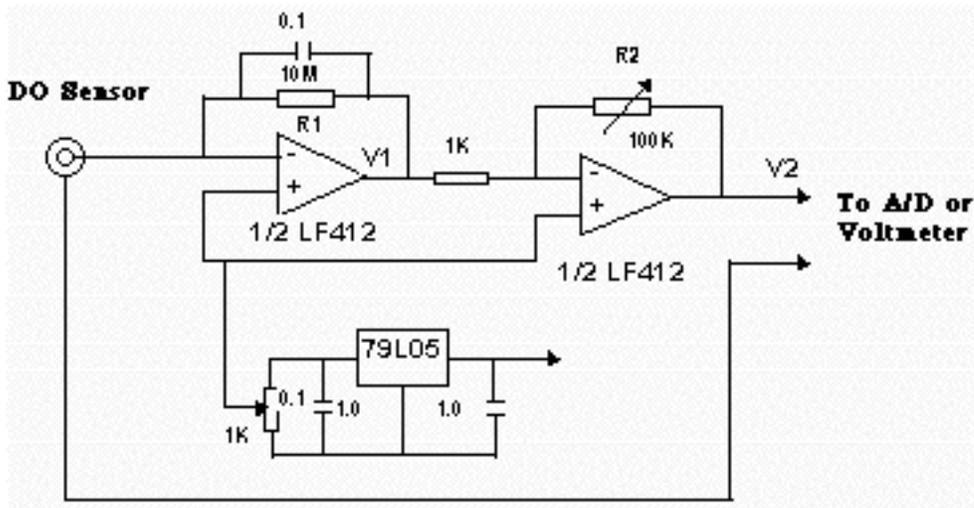
Fig. 2.4. Circuit for current to voltage conversion and application of polarization voltage.
