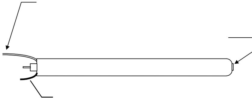
**Step 8.** Connect the copper wire to the center pin of BNC connector; connect the Ag/AgCl wire to the outer body of BNC by soldering.
