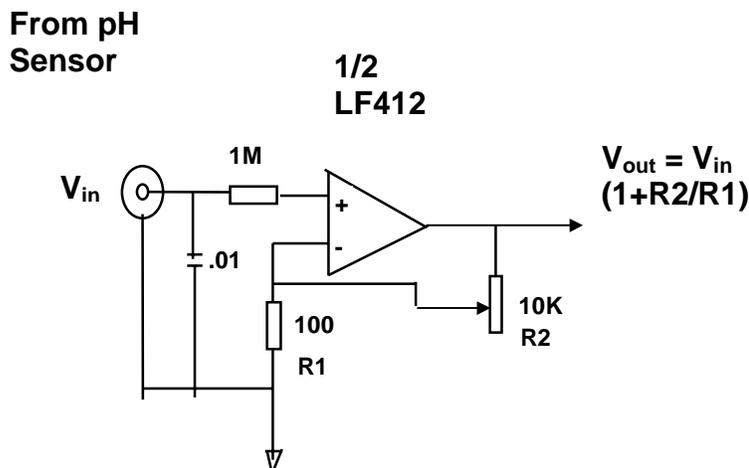
**Fig. 2.18. Signal conditioning circuit for potentiometry.**
