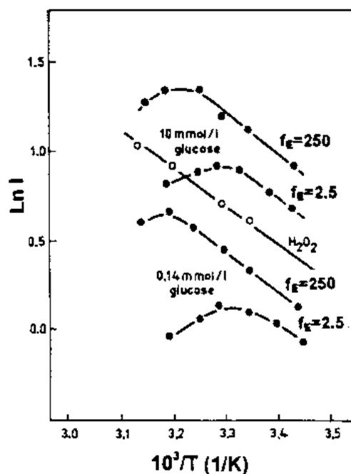
Fig. 4.7. Effect of temperature on sensor output.
