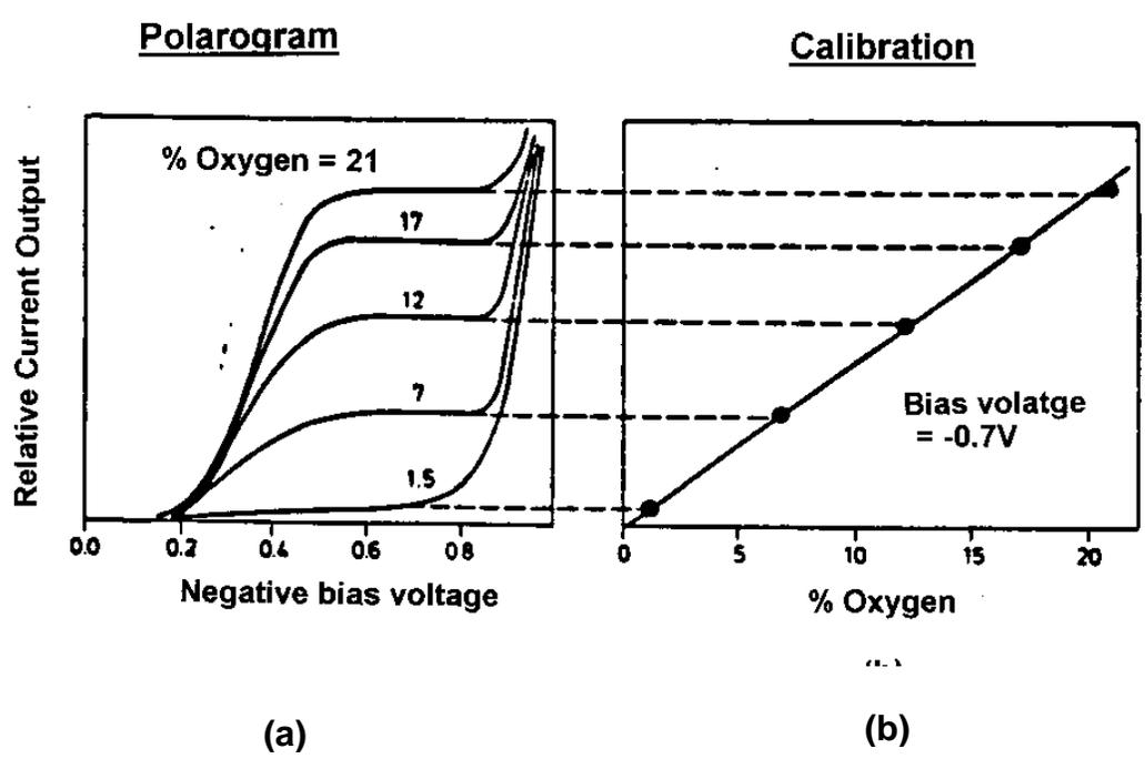
Fig. 2.2. (a) Current-to-voltage diagram at different oxygen tensions; (b) calibration obtained at a fixed polarization voltage of -0.6V.
