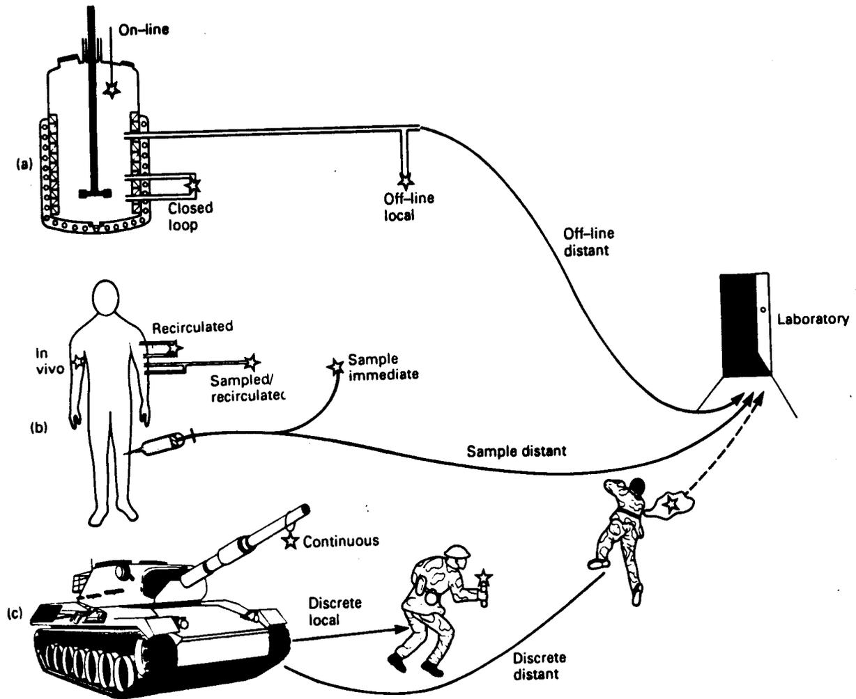
Fig. 1.7. Comparison of sensing modes: (a) bioreactor; (b) clinical applications; (c) military or environmental monitoring.
