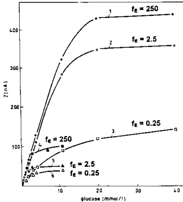
Fig. 4.5. Sensor output as function of glucose concentration.
