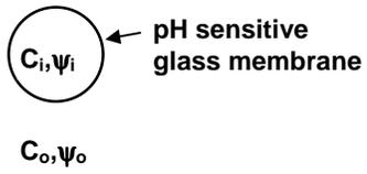
Fig. 2.15. Glass membrane electrode for pH measurement.
