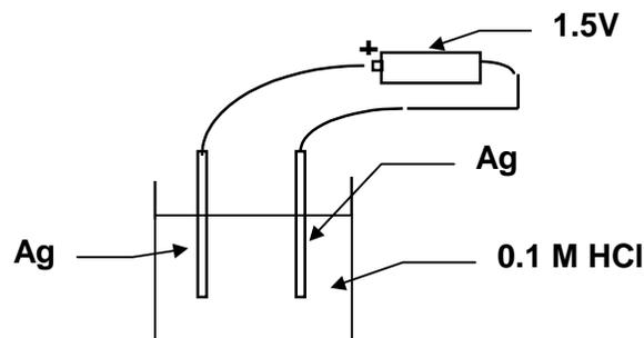
When the chlorination is done properly, the wire will have a brownish coat on it.
