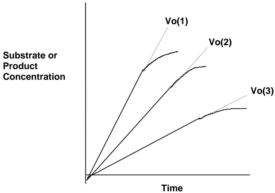
Fig. 3.5. Determination of initial rates at different substrate concentrations.
