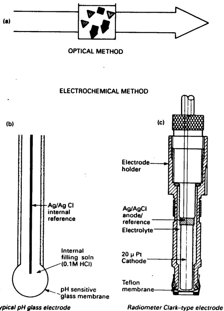
Fig. 1.11. Three conventional transducers used for biosensor development: (a) photometric; (b) potentiometric (based on pH sensor); (c) amperometric (based on Clark oxygen sensor).
