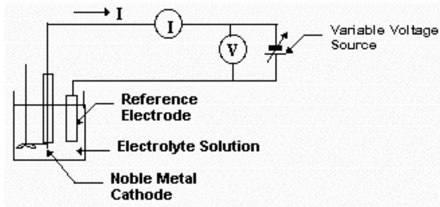
Fig. 2.1. Setup for polarography.
