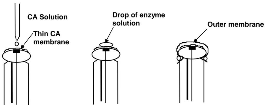
**Fig. 4.2. Glucose biosensor by physical adsorption of enzyme.**
