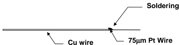
**Step 2.** Clean the Pt wire (just the Pt wire portion, not the Cu wire) by dipping in a 1:1 concentrated nitric and sulfuric acid solution. Wash with DI water.
