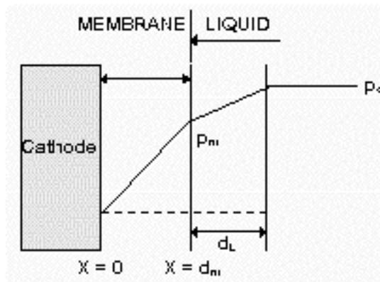
Fig. 2.8. Two layer model for DO sensor.
