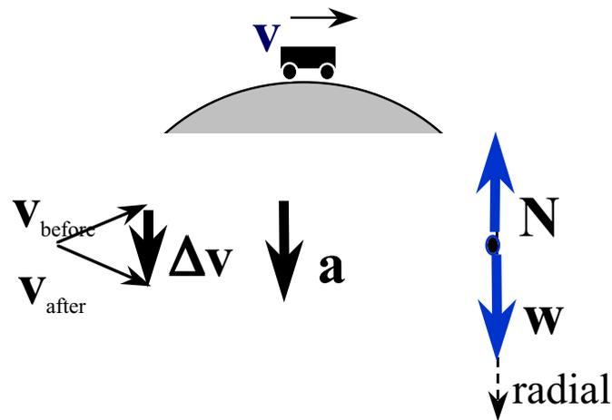
$$(40 \text{ kg})(9.8 \text{ m/s}^2) - N = (40 \text{ kg}) [(8 \text{ m/s})^2 / (10 \text{ m})]$$
